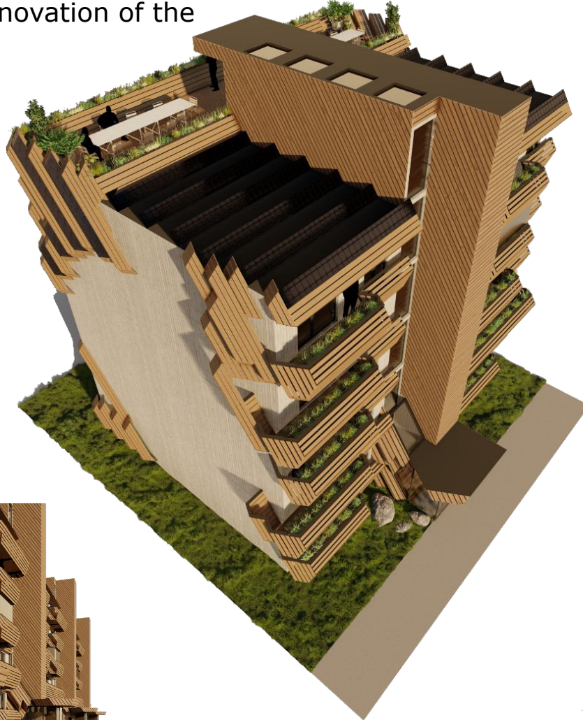
New access. A plug-in elevator and stair module with roof access
